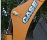
Large box-section structures with thick, multi-plate fabrications, castings, and forgings are used in high-stress areas such as the boom nose, boom foot, boom cylinder, and stick foot to improve durability.
